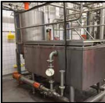
Steam injection **liquorice dissolver** with buffer tank
