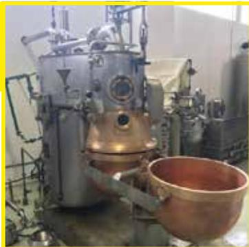
**Bosch 126E** solvomat is an automatic metering, dissolving and pre-cooking machine
