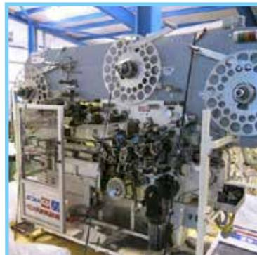
**ACMA GD ACX-5E** is a high speed stick gum wrapping machine and is complete with SF-1 breaker/feeder, with Allen Bradley Panelview 900 HMI. The wrap for the single piece is an inner wrap with an outer band
