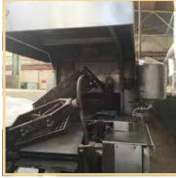
**Hebenstreit** wafer oven, gas fired automatic wafer baking oven
