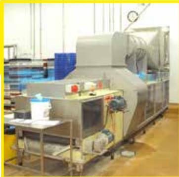
**Grading Machine** designed to separate oversized, undersized and precise sized pieces.
