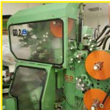
**GD 1001** high speed double twist wrapper for candy. Set on 24 x 15.5 x 10mm. Up to 1,000 p/m
