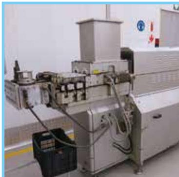
**Bosch** ball gum line that includes **WEF1120** extruder, **WAK0046** gum balling machine and **WSC1200AE** cooling tunnel
